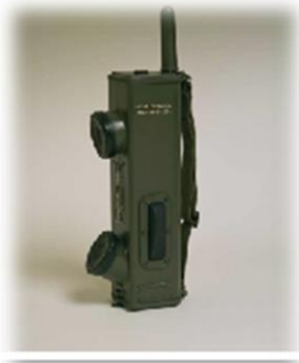
Galvin Manufacturing Corporation (later Motorola) Handie-Talkie SCR536 portable two-way radio, circa 1940.
